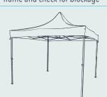
Adjust the height of the tent using the extendable legs. To do this, press the button (A) and lift the upper part of the leg (B). The lower part must slide by itself (C).
